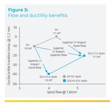
POTENTIAL PROCESSING BENEFITS USING LNP™ EXL COPOLYMER RESINS (depending on tool design):
