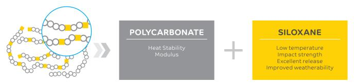
The EXL copolymer structure combines the best of PC and siloxane properties, resulting in a significant improvement vs. standard PC and PC blends. The siloxane forms a chemical link in the PC backbone to provide outstanding low temperature impact performance. Since silicone is relatively unaffected by heat or humidity under typical aging conditions, the materials retain their properties longer than standard PC.
