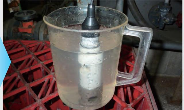
\*The treated water in the photo is not a supernatant (the top clear layer of liquid above solid residue after precipitation, etc.). It is water extracted during aeration stirring. A key characteristic of Aquablaster is that it even treats suspended solids. Please feel free to [tour a facility in operation](#). (\*No activated sludge used)
